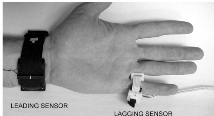
**Figure 2.** Wrist and Finger PPG Sensors [21]
