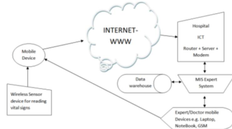
Figure 1. Wireless sensor framework for Hypertension [12]
